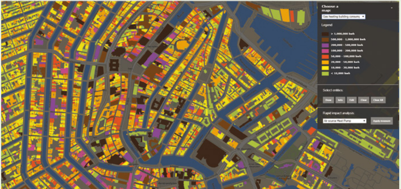
Screen shot of the Decision Support Tool, showing the gas usage of individual buildings in the city centre of Amsterdam
